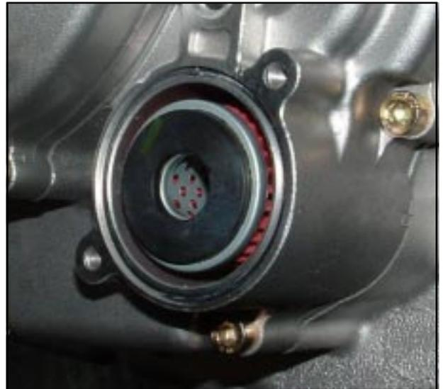
Remount the cover, being careful to the O-Ring and to insert the filter cover nose correctly into the hole of the filter cartridge. Greasing the O-Ring with a small amount of grease helps to keep it in its seat when assembling.
