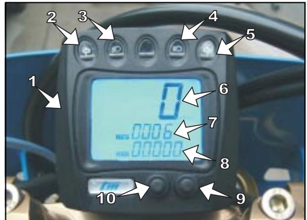
The instrument unit is the Km/h but it can be easily changed in Mph in the following way: press and hold the "SET" button, while holding it press once the "MODE" button.
